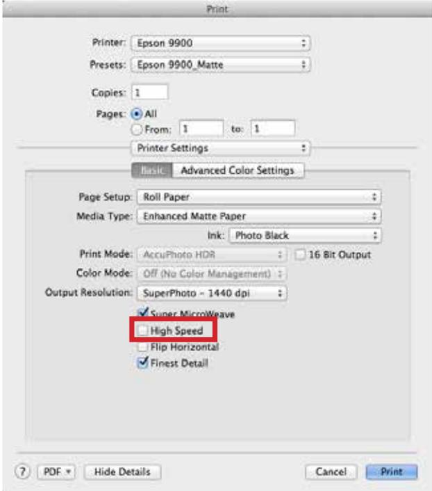
V. Uncheck “High Speed” in Printer Settings
